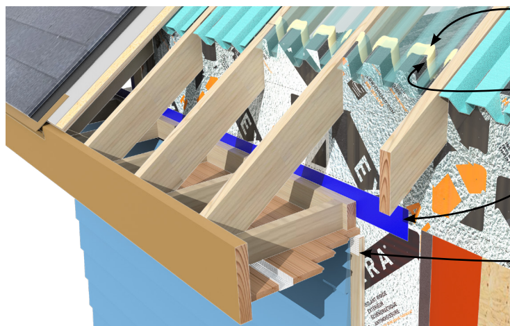
Roof transition detail: Exterra extending to underside of roof baffles
