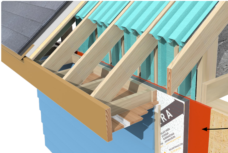
Roof transition detail: Exterra extending flush to top sill plate
