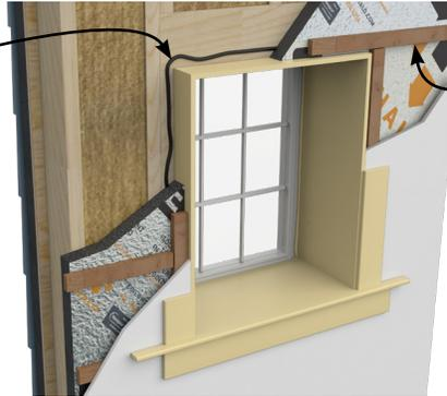
Optional wood strapping over Interra provides an air space needed to reflect heat back to the interior of the building, reducing heat loss.
